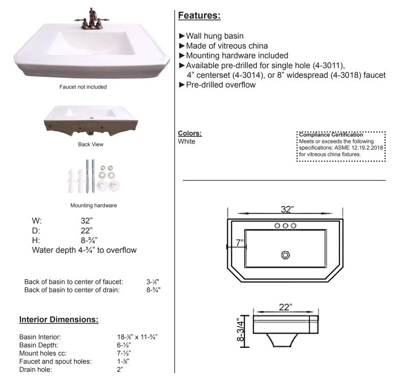
Dimensions of fixture are nominal and may vary within the range of tolerances established by ASME Standard A112.19.2.2018. Dimensions and specifications subject to change without notice.
